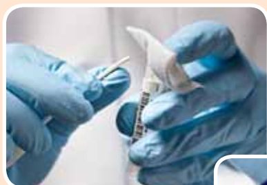
Break swab in sample tube
