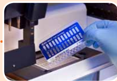
Load PCR cartridge(s)
